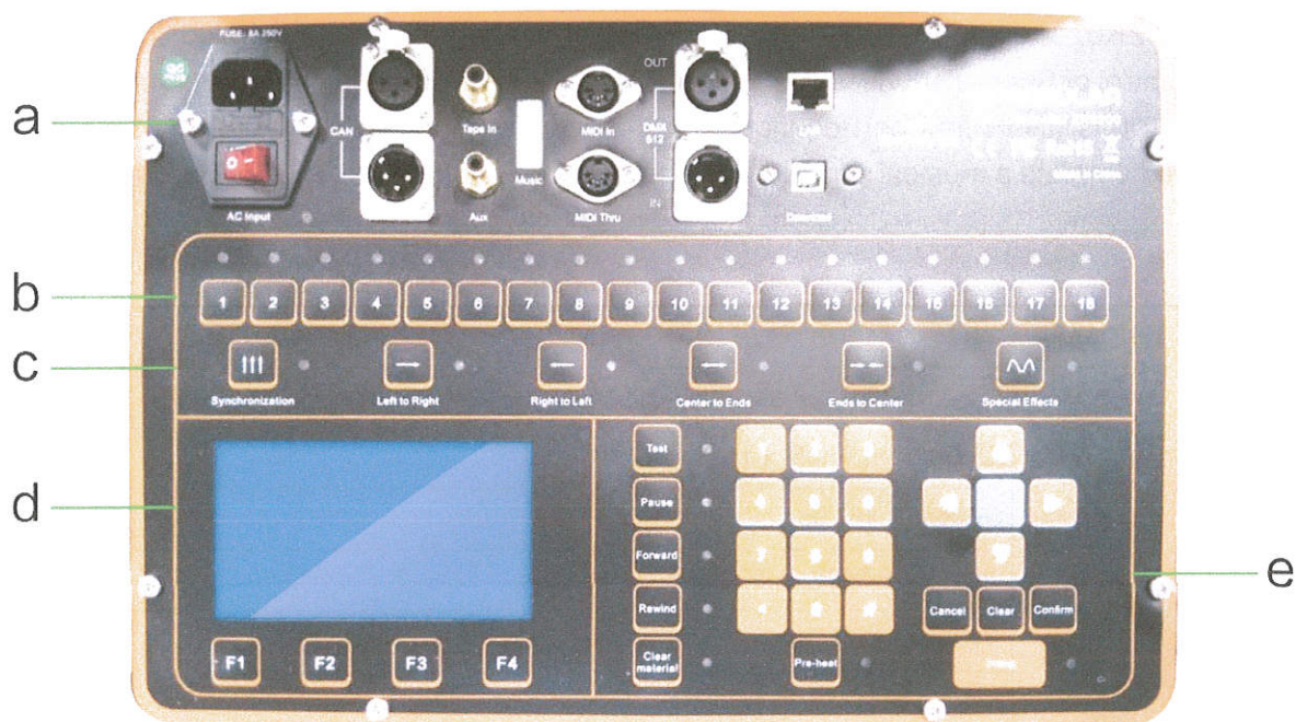
Controller Operation Panel
